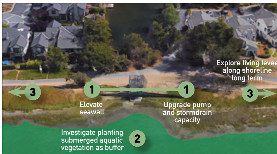
Alameda's resilience plan explores options for spots vulnerable to sea-level rise such as this lagoon inlet on Bay Farm Island.
